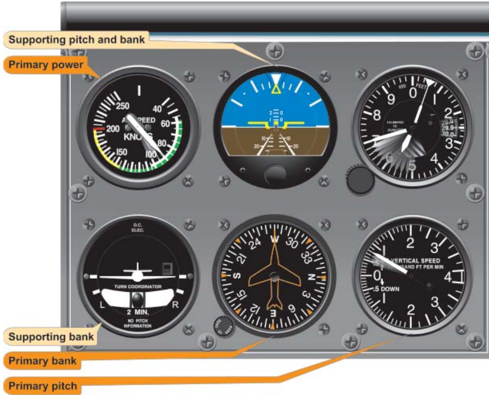
Figure 5-28. Airspeed Low and Vertical Speed High—Reduce Pitch.
