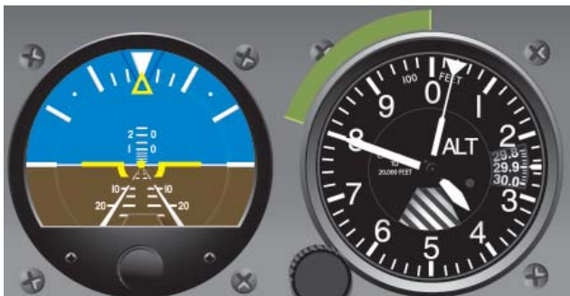
Figure 5-11. Altitude Error, Greater Than 100 Feet.
