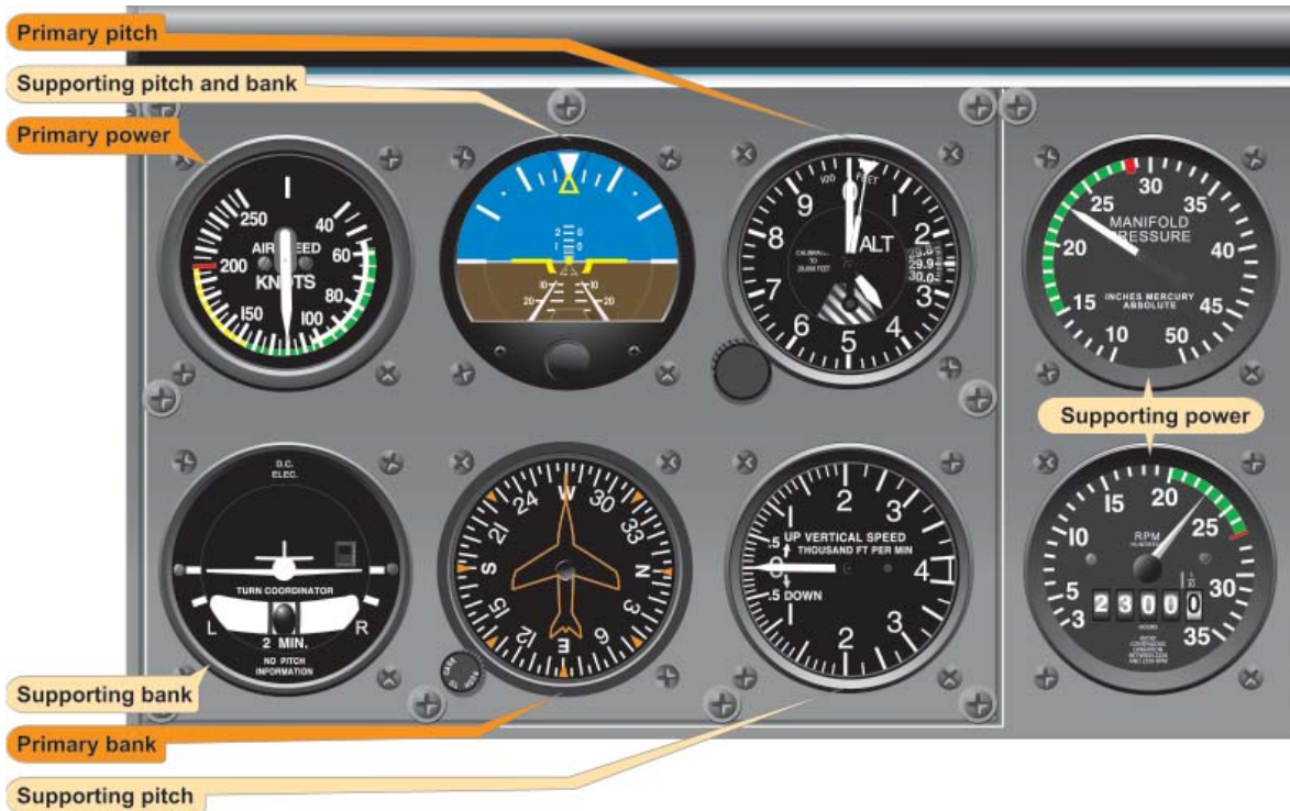
Figure 5-22. Straight-and-Level Flight (Normal Cruising Speed).
