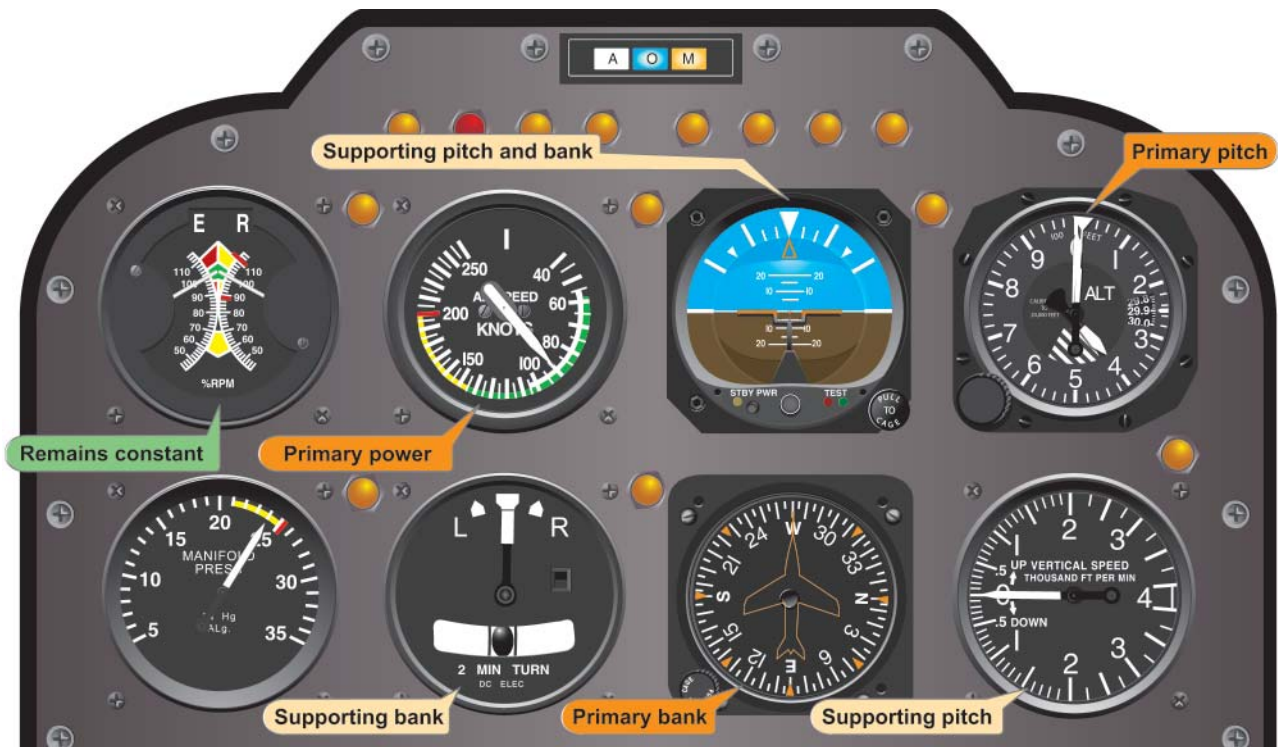
Figure 6-9. Flight instrument indications in straight-and-level flight at normal cruise speed.
