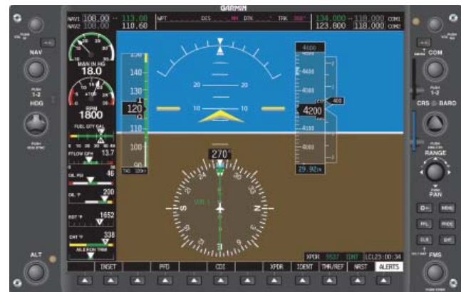
Figure 5-51. Pitch Illustrated at 10°.
