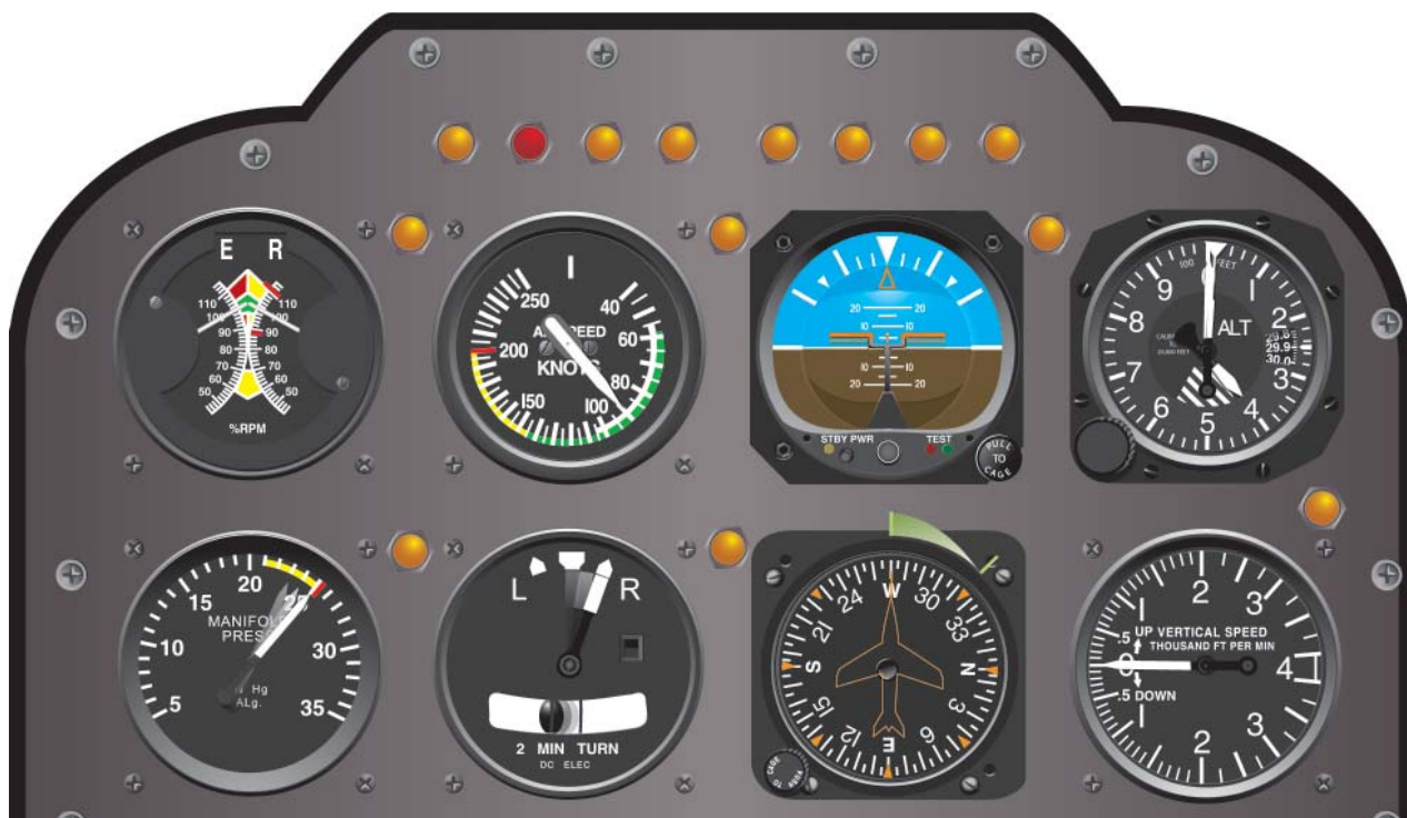
Figure 6-7. Flight instrument indications in straight-and-level flight with power increasing.
