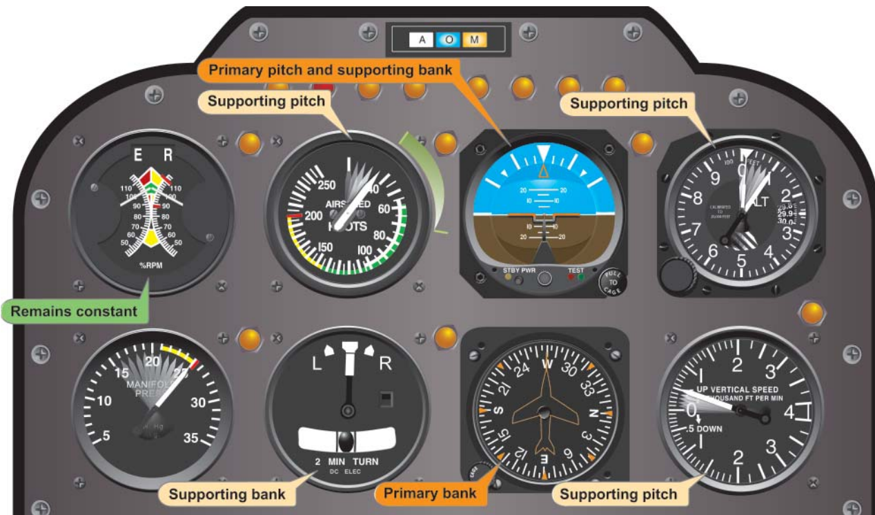
Figure 6-16. Flight Instrument Indications During an Instrument Takeoff.
