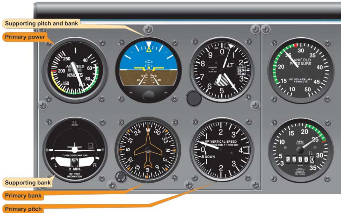
Figure 5-27. Stabilized Climb at Constant Rate.
