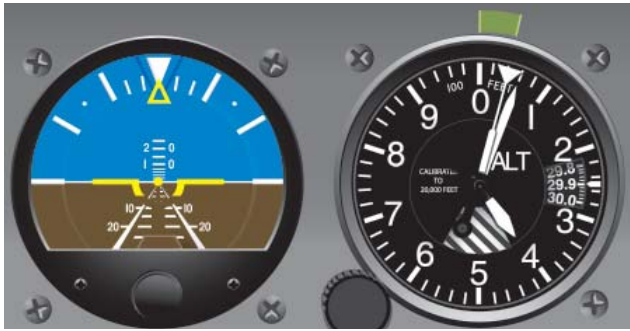
Figure 5-9. Altitude Error, Less Than 100 Feet.
