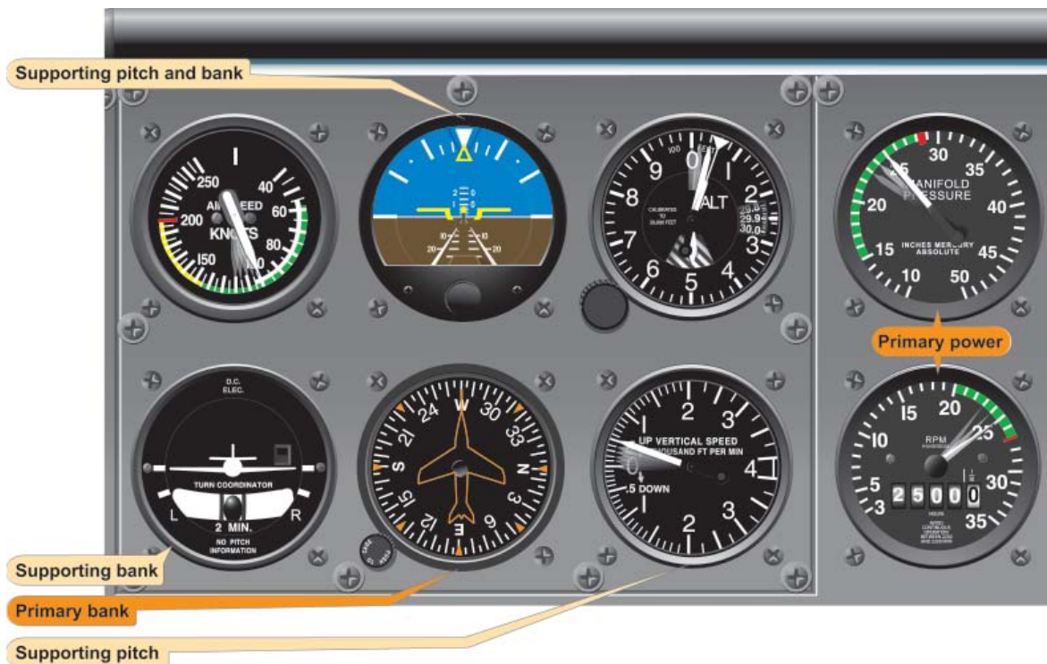
Figure 5-25. Climb Entry for Constant Airspeed Climb.
