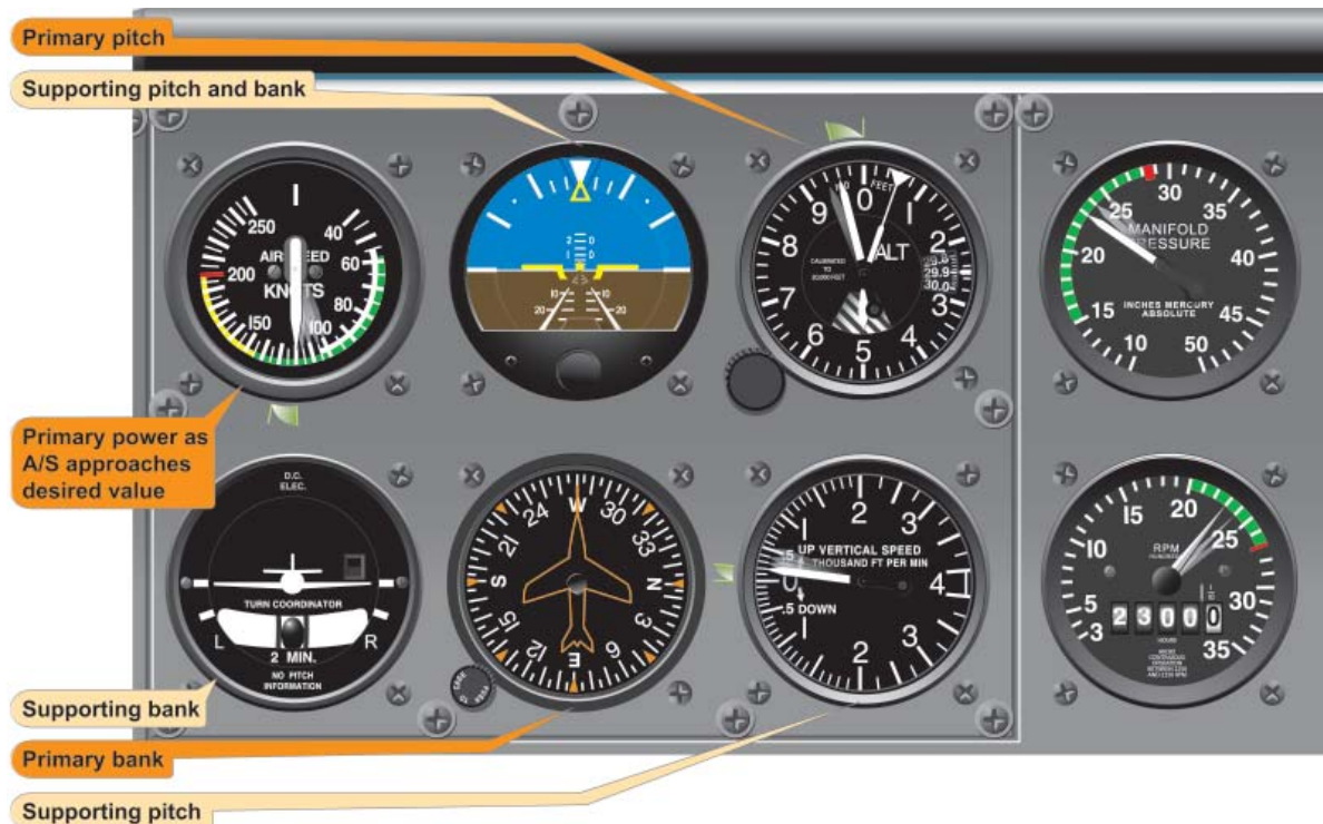
Figure 5-29. Level Off at Cruising Speed.
