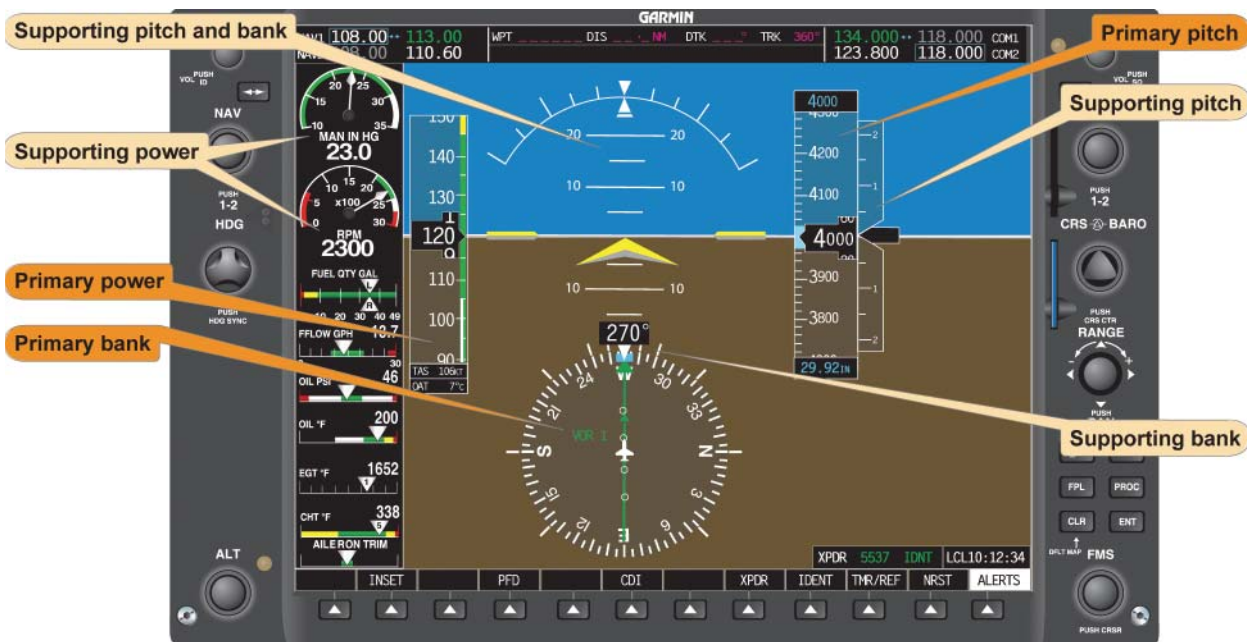
Figure 5-57. Straight-and-Level Flight (Normal Cruising Speed).
