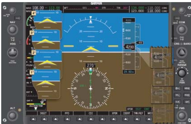
Figure 5-50. Pitch Indications for Various Attitudes (1° through 5°).
