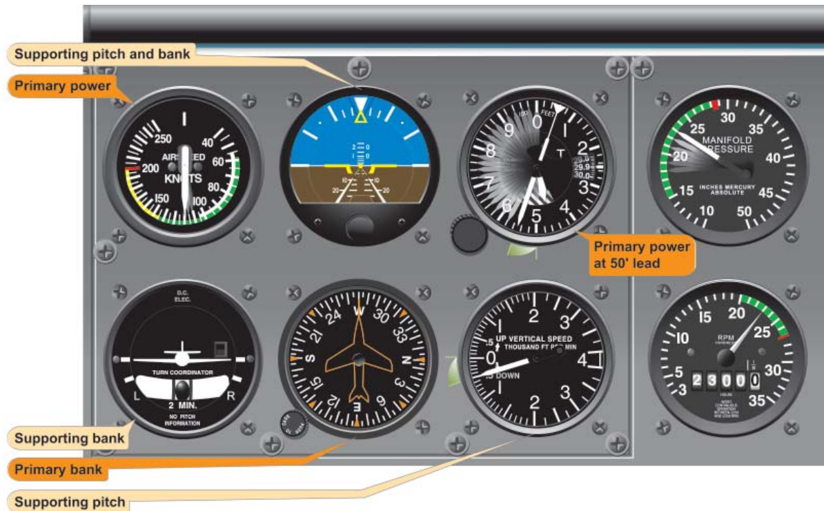
Figure 5-32. Level Off at Descent Airspeed.
