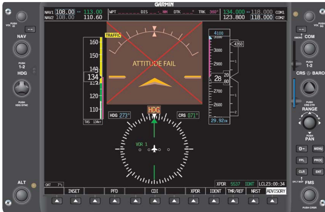
Figure 5-73. AHRS Unit Failed.
