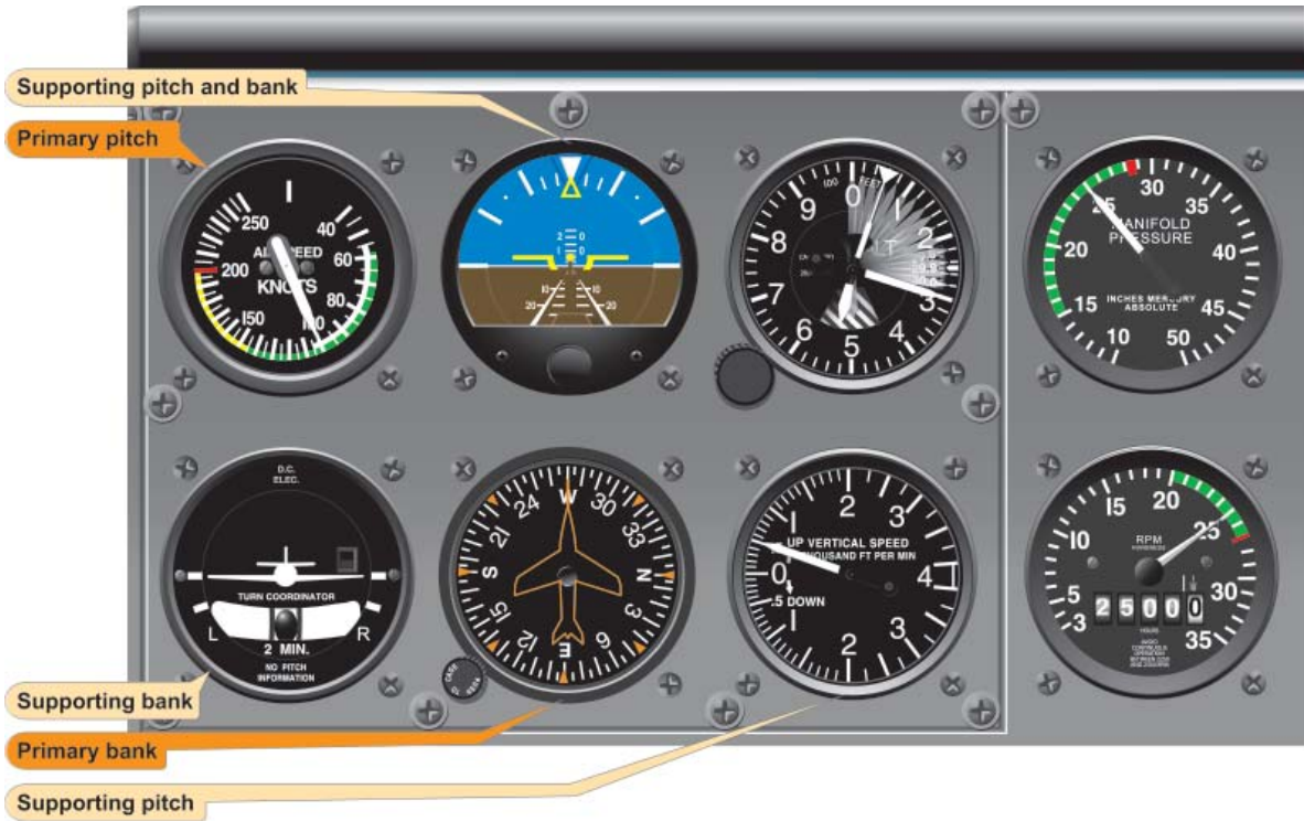
Figure 5-26. Stabilized Climb at Constant Airspeed.
