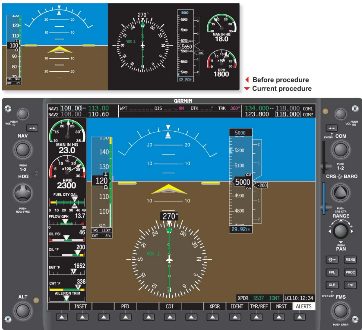
Figure 5-66. The top image illustrates a reduction of power and descending at 500 fpm to an altitude of 5,000 feet. The bottom image illustrates an increase in power and the initiation of leveling off.
