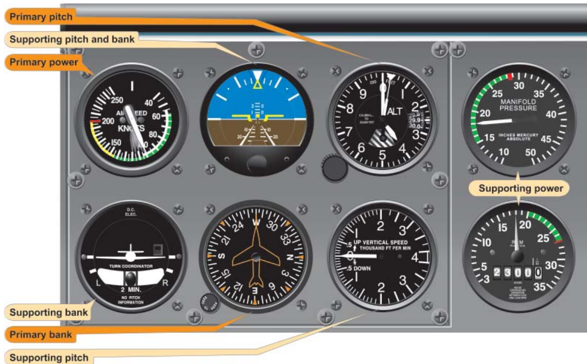
Figure 5-24. Straight-and-Level Flight (Reduced Airspeed Stabilized).
