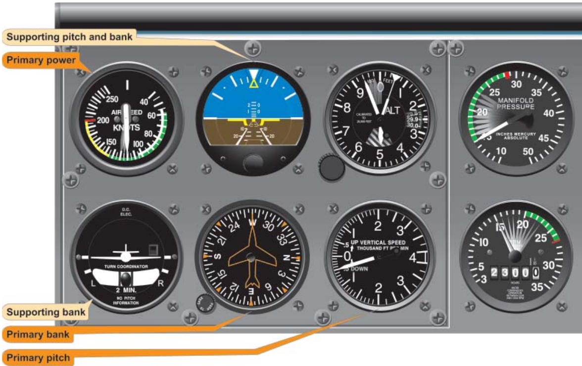
Figure 5-30. Constant Airspeed Descent, Airspeed High—Reduce Power.
