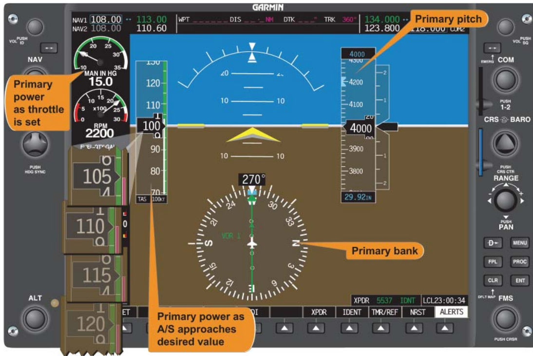
Figure 5-58. Straight-and-Level Flight (Airspeed Decreasing).
