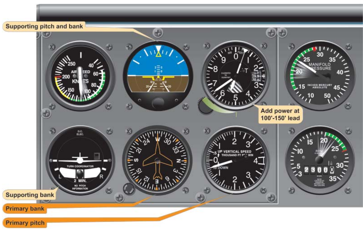
Figure 5-31. Level Off Airspeed Higher Than Descent Airspeed.
