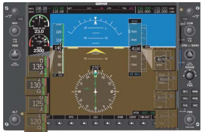
Figure 5-56. Figure shows both an increase in speed and altitude where pitch adjustment alone is insufficient. In this situation, a reduction of power is also necessary.
