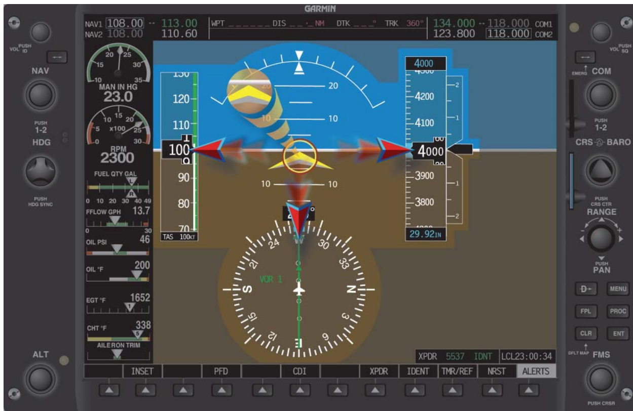
Figure 5-60. Cross-check Supporting Instruments.
