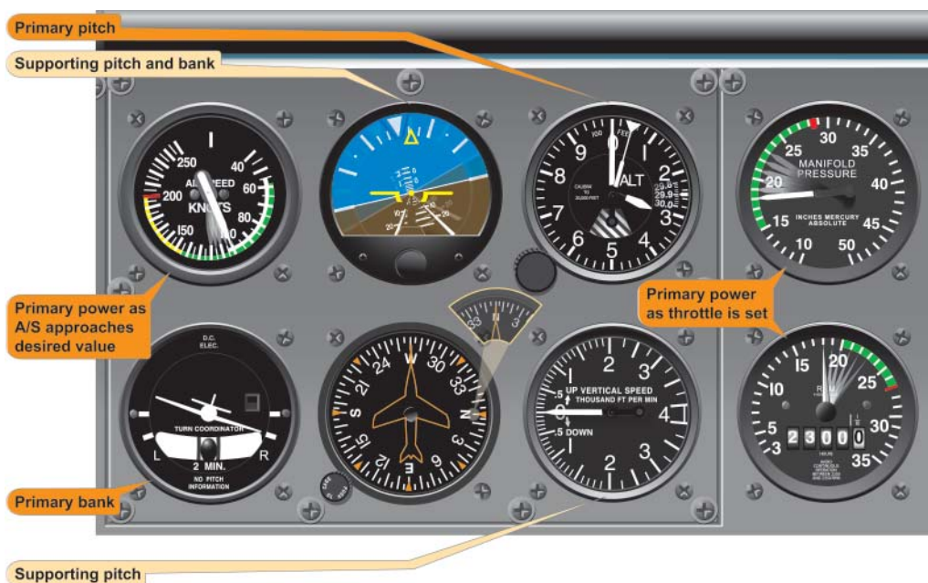
Figure 5-38. Change of Airspeed During Turn.
