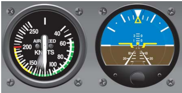
Figure 5-15. Constant Power Plus Increased Pitch Equals Decreased Airspeed.
