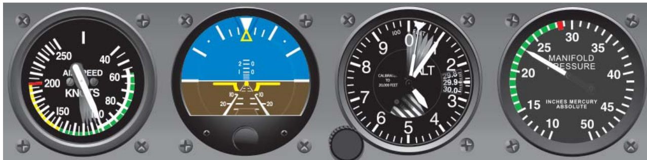
Figure 5-20. Airspeed Low and Altitude High—Lower Pitch.
