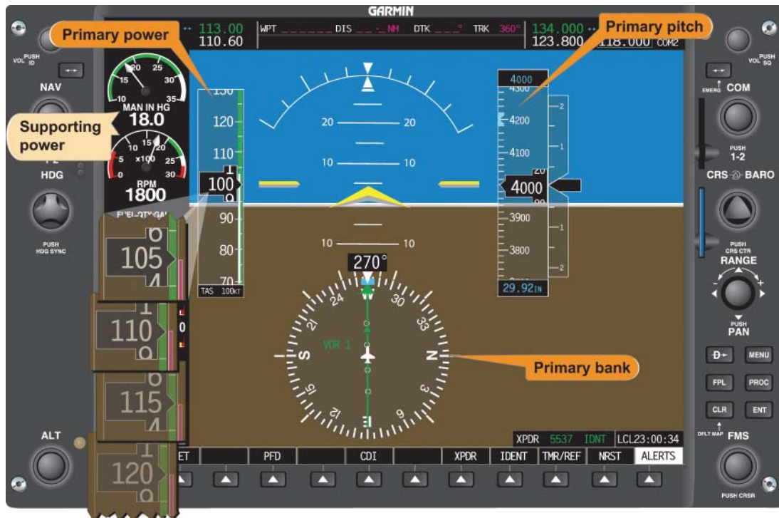
Figure 5-59. Straight-and-Level Flight (Reduced Airspeed Stabilized).
