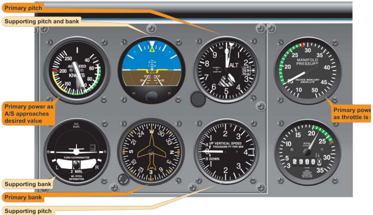
Figure 5-23. Straight-and-Level Flight (Airspeed Decreasing).
